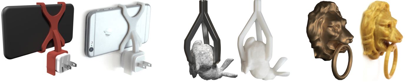
Figure 1: We introduce a method for designing coupling behaviors between an arbitrary compliant structure and an arbitrary rigid object. Resulting structures exhibit the desired coupling behavior such as ease of engagement/disengagement and grip.
