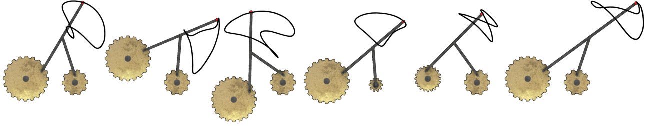
Figure 3: The driving mechanisms we use as building blocks can generate a continuous space of widely different motions. To generate optimized assemblies that best match an input motion, we first perform a coarse exploration of the space of possible motions for each mechanism, followed by a continuous parameter optimization.
