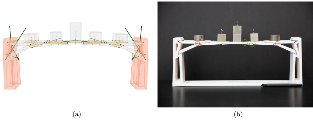
Fig. 16. (a) Bridge in its final configuration and subjected to additional loads. (b) The span of the 3D printed model is 40 cm, the net mass of the bridge is 319 g, while the mass of the external loads is 1208 g. The red circles denote two sharp wedges designed to guarantee that the two external elements are in the right position. (For interpretation of the references to colour in this figure legend, the reader is referred to the web version of this article.)
