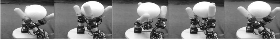
Fig. 3. To demonstrate the feasibility of our designs, we fabricated a hand with 3D printed parts scaled with regard to the embedded motors. This particular design is meant to rotate a 4 inch diameter ball 180° either way.
