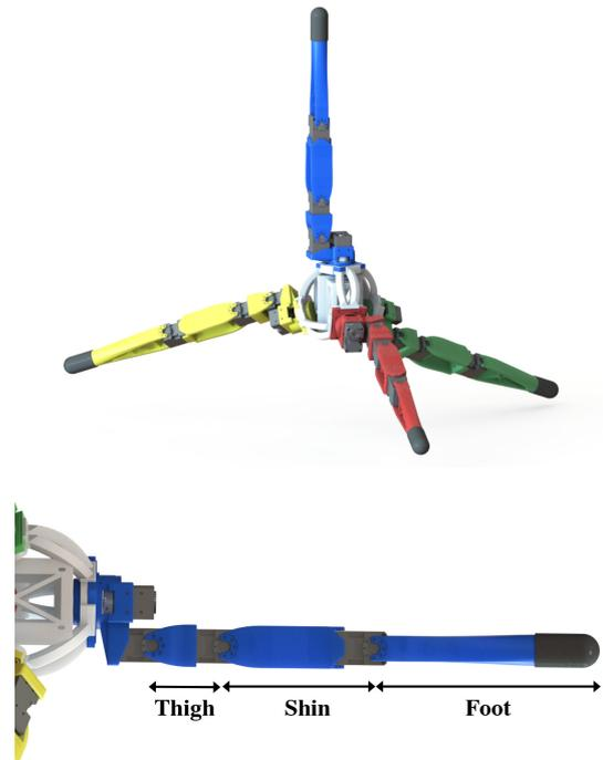
**Figure 15.** A spherically symmetric quadruped robot, *Tetrabot*. **(Top)** The zero pose of *Tetrabot* is similar to a tetrahedron. **(Bottom)** Each leg has four DoFs including one yaw joint and three pitch joints.
