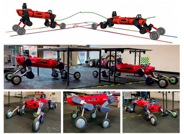
Figure 12. Motion composition of three offline trajectories based on the interactive TO in Section 4.2. The upper visualization shows the torso and end-effector trajectory of the composed trajectory m(t) . Here, the robot executes two ducking motions with a duration of 2 s each, connected by a 90° turn with a duration of 1.7 s and two repositioning transitions. (see lower images).
