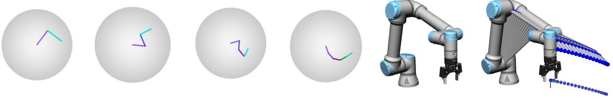
Fig. 4: **Left to right**: Planar IK for n-link serial robots  $n = 2$  to 5. IK for UR5, Kinematic TO for UR5
