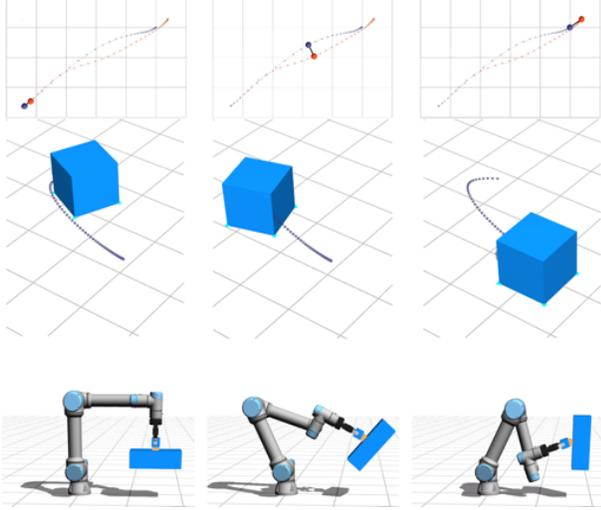
Fig. 7: **Top Row:** Dragging a point mass (purple) towards the origin. **Middle Row:** Repositioning and reorienting a rigid body box sliding over a frictional surface. **Bottom Row:** Reorienting a rigid body box with a flexible attachment.
