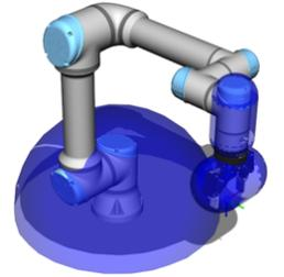
Fig. 8: Collision primitives
