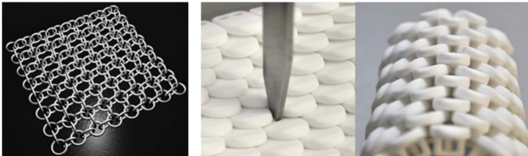
Additively manufactured chain mail (left) and laser sintered articulated stab-resistant armor (right)
