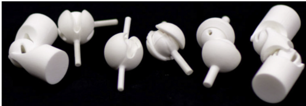
Articulated joints produced using selective laser sintering (SLS)
