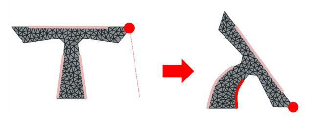
say the control input p are the contacted lengths of cables in a soft robot... given a target pose  $\widetilde{x}$ , what is the optimal control  $p^*$ ?
