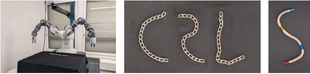
Fig. 7: We validate the generated trajectories on an ABB YuMi robot (left). Letters from the “Computational Robotics Lab” logo (center) formed with a steel chain and a “S”-shape (right) formed with a cotton cord.
