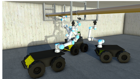
Fig. 1: Render of a multi-robot system cooperatively installing a prefabricated element on a construction site.
