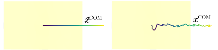
Figure 3. A top-down view of the Puppy 's target center of mass trajectory \hat{\mathbf{x}}^{\text{COM}} (left) for walking in a straight line, and the corresponding simulated center of mass trajectory \mathbf{x}^{\text{COM}} made with optimal control signals \mathbf{u} (right). In both cases the robot's body is shown at its starting position in yellow. Note that the short grey portion at the beginning of the simulated trajectory corresponds to the preparatory phase of motion, discussed in Section III-B.
