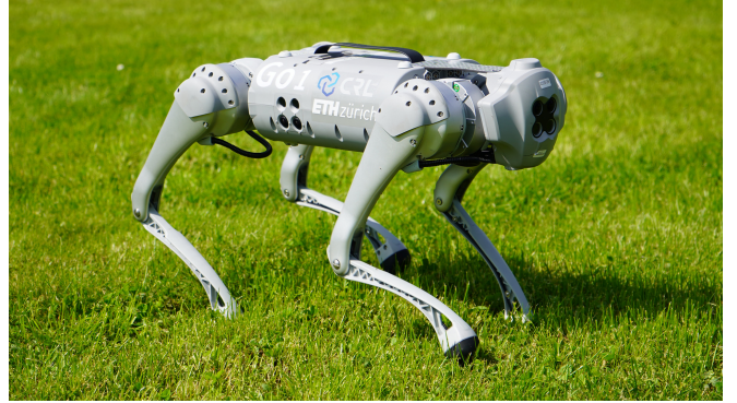
Fig. 1: The quadruped robot Unitree Go1 executing the target gait pattern trot while walking on a grass field.
